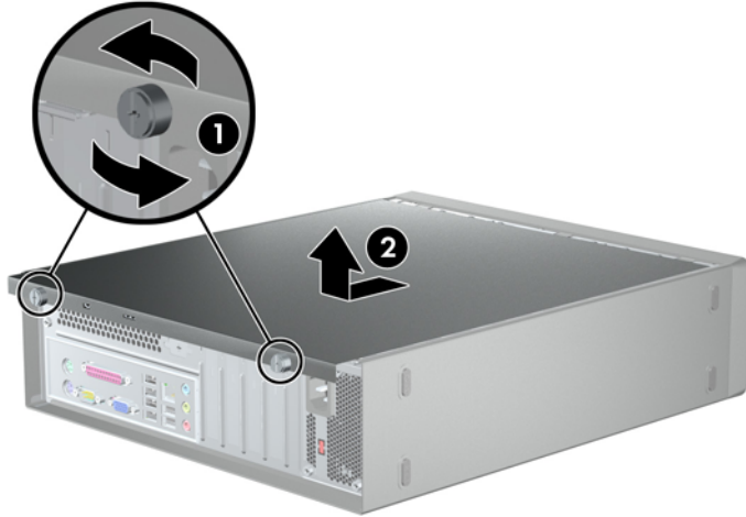
Figure 7-1 Removing the Access Panel
